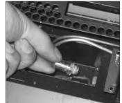
Figure 22: Orifice Replacement.
